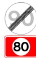
UC57: End of local speed limit subpanel
