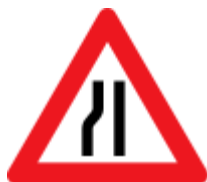
A43.2: Road narrows left side
