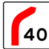
E41: Recommended max speed on exit
